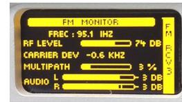
Figura 11: Pantallas del receptor FM
