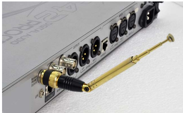
Fig. 6. Digital receiver antenna at the rear side of the audio processor.
