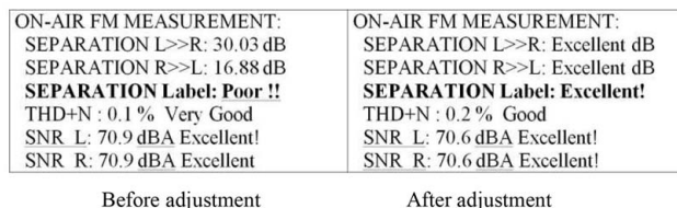
Fig. 10. Audio quality report of a radio station located at Pilar, Buenos Aires, measured with software version 2.xx.
