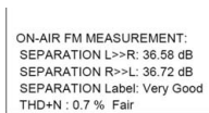
Fig. 9. Audio quality report of the Fig. 8 radio station after a remote adjustment using a Monitored Audio Processor.
