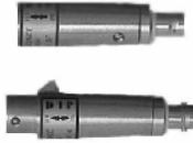
**AES-3 output** has a resolution of 24 bits with a samplerate selectable between 48/96 KHz (see “3.2.2 – Output Setup”). The connector is male XLR.
