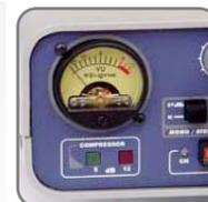
**An excellent needle VUmeter** measures true peak signal and can be perfectly seen at full sunlight.
