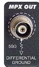
**The old problem of** the humming due ground loops does not exist in our processors, because the **MPX** out is differential and provides **45 dB** of hum cancellation.
