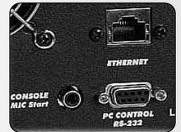
At the same time, the **RS232 / USB** interface from PC, allows the air automation software controlling the 562 in order to change to one of the 30 stored programs that best fit the musical style. The best processing setting for Jazz is not the same that for Rock & Pop or promotional Ads.
