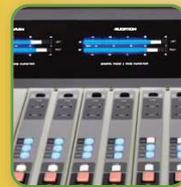
A complete turret with 4 Dual VUmeters, Timer, Clock and Phase Vector to know the degree of deepness of stereo sound.
