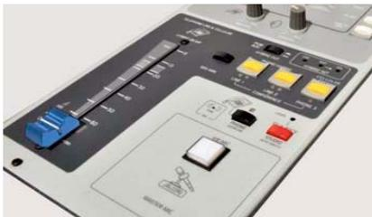
Phone call rings at the console speaker with flashing blue light. It can be attended from the console panel. The console also allows the use of telephone sets to manage the communications from the Production people or by the operators.
