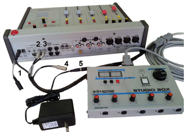
Figure 2: The DB9 connector was replaced by RJ45 in new models
