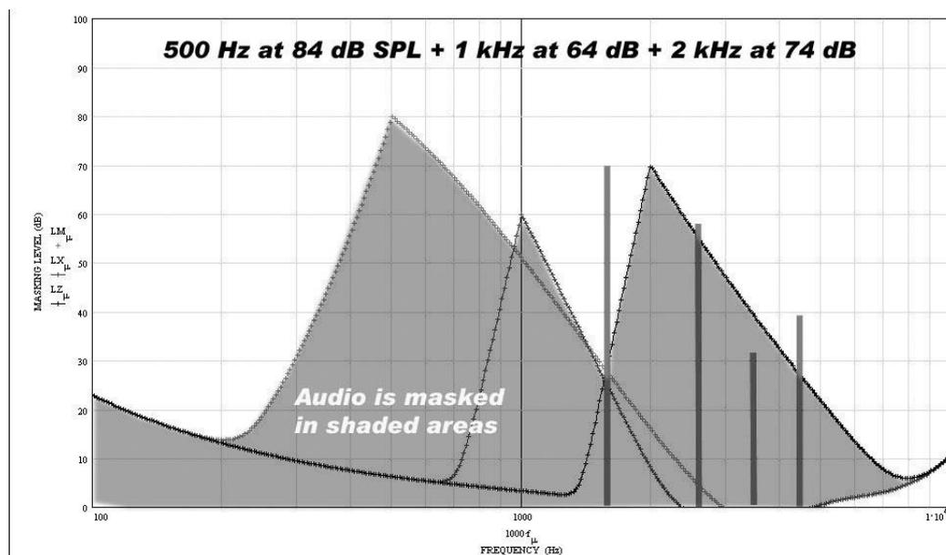
FIG 5 Masking 500 Hz clip, when 3 bands are present
