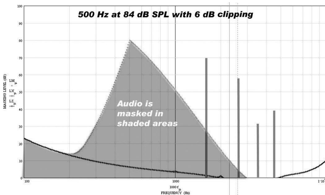
FIG 4 Harmonics of the 500 Hz clipped wave
