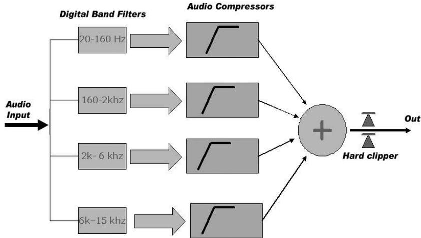
FIG 1 Block Diagram of multiband compressor
