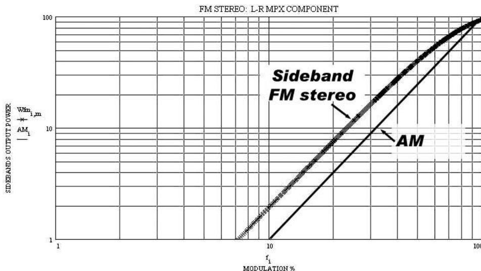
FIG 11 FM stereo sidebands at 38 kHz sub carrier
