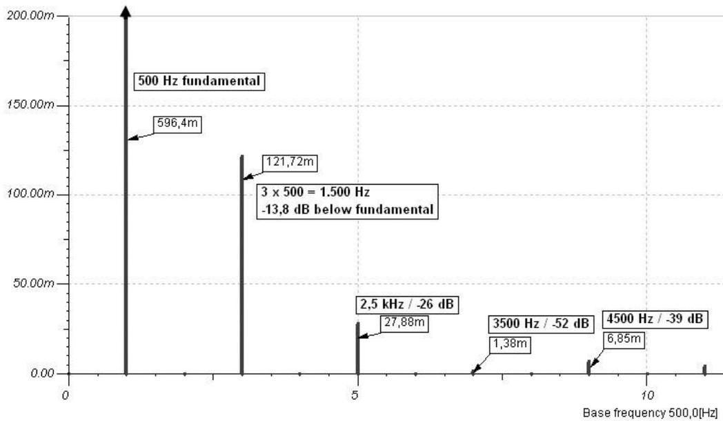
FIG 3 500 Hz, 6 dB clipping, harmonic spectrum
