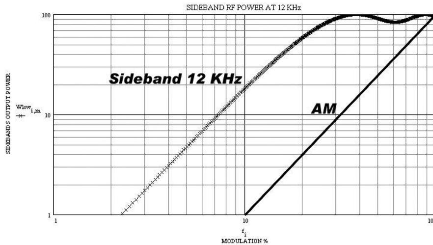
FIG 10 FM sidebands at 12 kHz modulation
